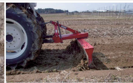
Fig. 1-b Removal of surface soil by earth moving equipment.
